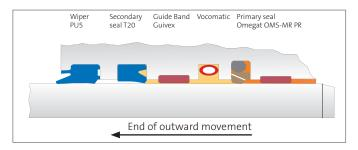
The Merkel Vocomatic has completely absorbed the volume of the drag oil. The pressure in the inter-space remains low compared to the pressure in the working area of the cylinder. The secondary seal is slightly activated only.
