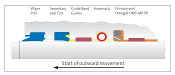
The primary seal covers the sealing function completely. The Merkel Vocomatic is relaxed.
