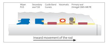
The pressure relief bore in the Merkel Omegat primary seal enables a flow of the drag oil back into the working area of the cylinder. This flow is supported by the restoring force of the compressed Vocomatic.
